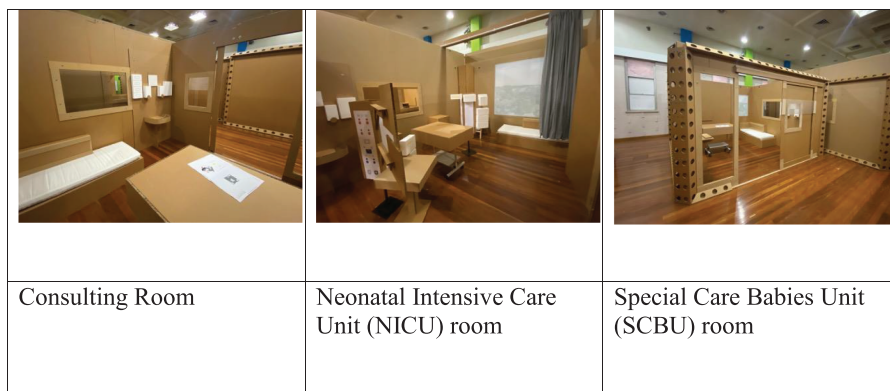
Figure 2: 1:1 Mock-ups of different room designs for the Adelaide New Women’s and Children’s Hospital
