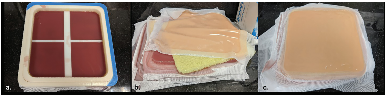
Figure 1: (a) Rectus abdominis layer curing within 3D-printed mould. (b) Collection of various tissue layers prior to final assembly. (c) Unmounted, fully cured product with overlying skin
